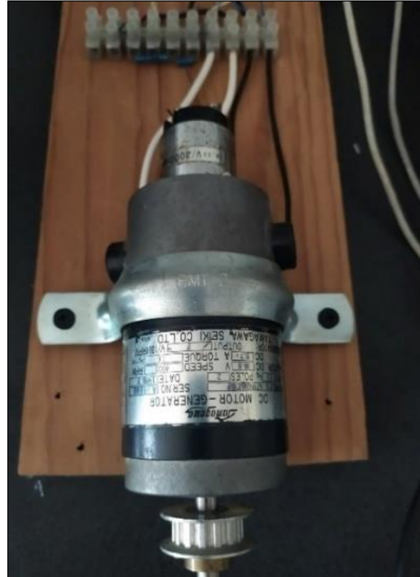
Figure 2: No-load direct current motor.
