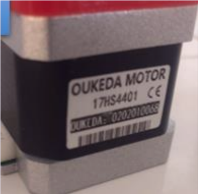
NEMA 17 motor 200 step stepper
