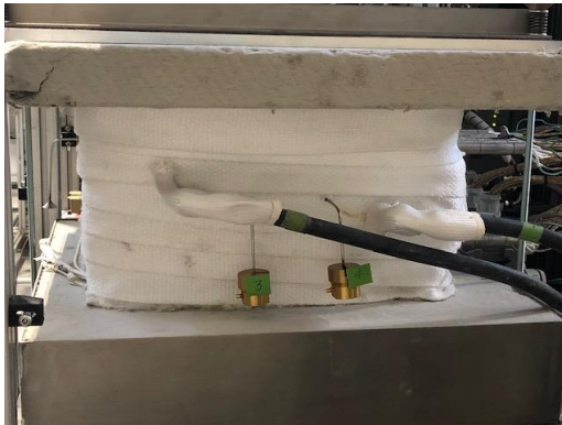
Fig. 2. Assembly of AE sensors 3 and 4 in the middle of the Stack.
