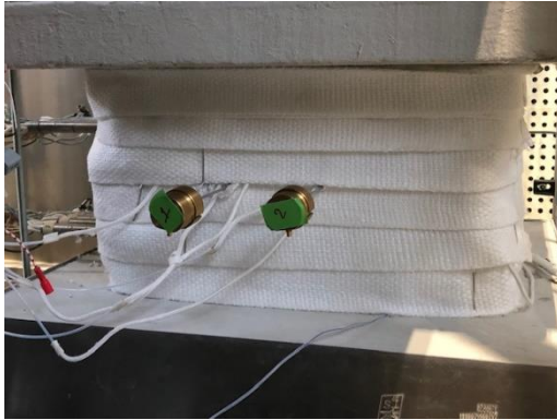
Fig. 1. Assembly of AE sensors 1 and 2 in the middle of the Stack.
