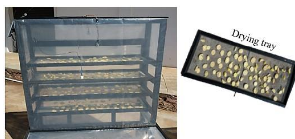
Figure 2 Guava drying chamber and drying trays
