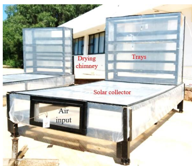
Figure 1 Mixed type rustic solar dehydrator
