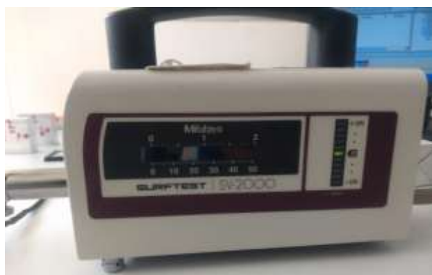
Figure 6 Mitutoyo SURFTEST SV-2000 roughness tester Source: Own Authorship
