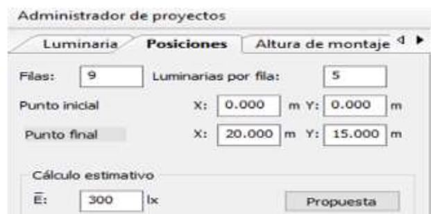
Figure 14 Average illumination level 300 lx. Source: Dialux
