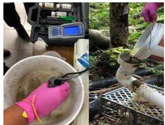
Figure 5 Preparation of organic waste and loading to biodigester Own Source
