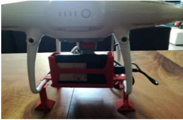
Figure 7 Connection of the multispectral sensor Source: Own
