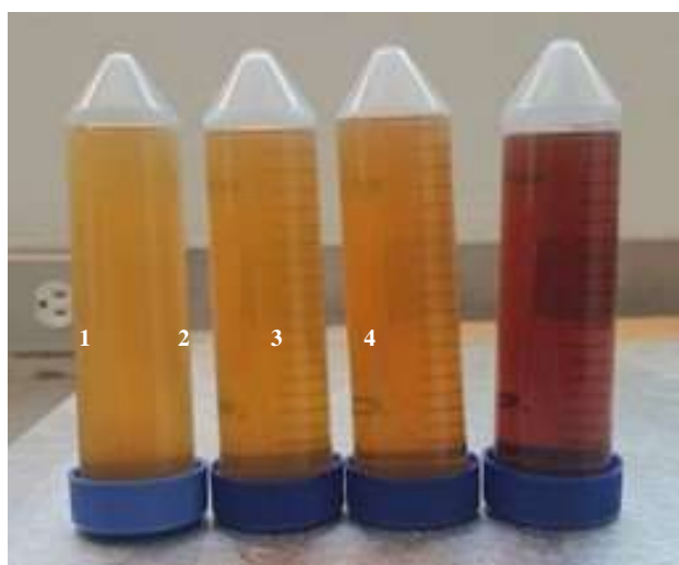
Figure 7 Filtered samples after biological treatment (1, 2 and 3) and physicochemical treatment (4)
