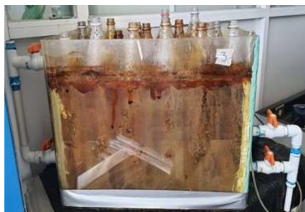
Figure 5 Biological reactor adaptation to the effluent with butyl acetate
