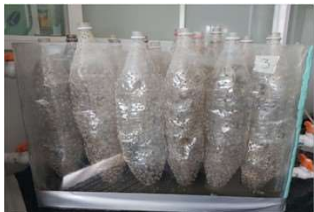
Figure 2 Fixed aerobic biological reactor prototype
