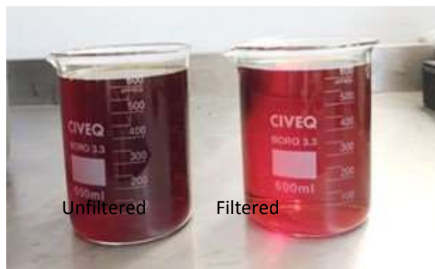
Figure 6 Physicochemically treated sample before and after filtration
