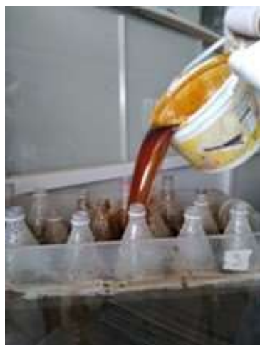
Figure 4 Biological reactor feeding with domestic wastewater and effluent with butyl acetate mixture
