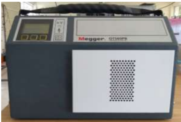
Figure 1 Schematic of an OTS60PB 70°C dielectric strength meter with a measurement range of 60 kV and a scale division of 1 kV
