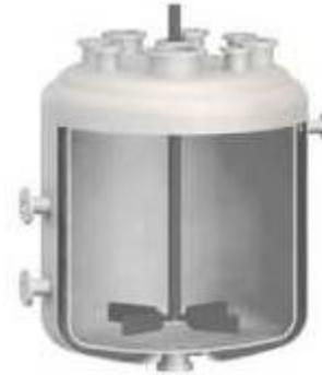
**Figura 2** Reactor batch
