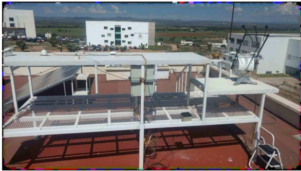
Figure 3 Zacatecas_04 Solarimetric Station of the National Solarimetry System
