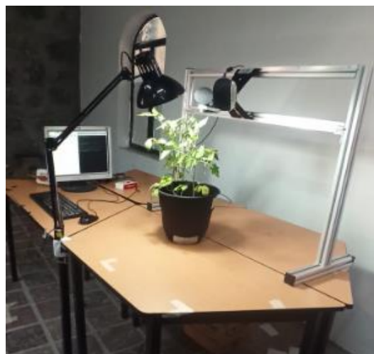
Figure 1 Image capture system hardware: camera, lamp and raspberry pi 3
