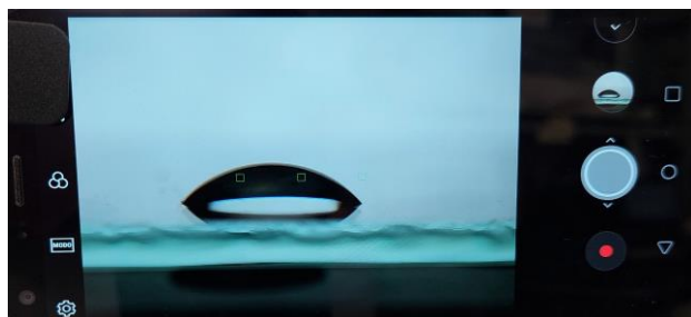
Figure 3 Drop of water photograph for contact angle measurement
