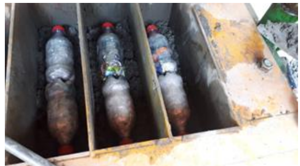
Figure 1 355 ml bottles of pet inside the block Source: Own elaboration
