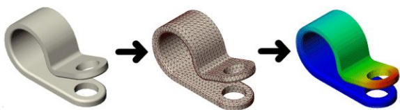
Figure 6 Element, mesh, and Stress intensity representation Source: (Solidwoks,2020) [3]
