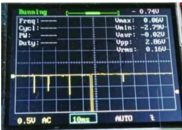
Figure 12 Non-inverted myoelectric signal processed by the EMG module Own Authorship
