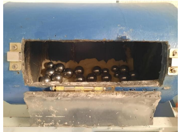
Figure 1 Illustration of the crushing and grinding of silicon rock
