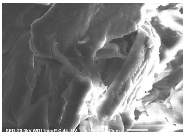
Figure 6 PET with heat treatment. 1500X
