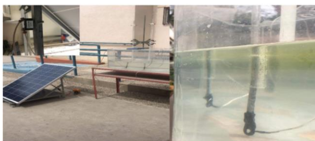
Figure 3 Experimental arrangement A) Experimental arrangement of the seawater electrolysis process in operation using a PV panel. B) On / Off toggle switch connected between the PV panel and the graphite electrodes. C) Graphite electrodes positioned inside the pipettes in the acrylic with seawater in the electrolysis process
