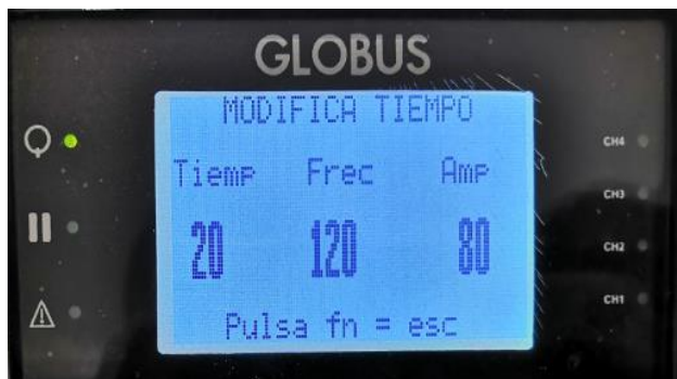
Figure 7 Programming of the electrostimulator: TENS high frequency Source: Self Made
