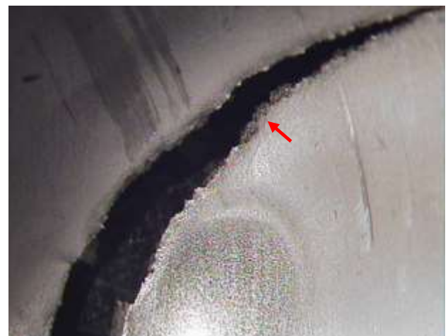
Figure 2 Internal surface of the stamped and cracked component after the second process step. The crack located in the lower radius of the component can be observed
