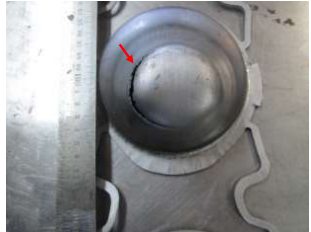
Figure 1 Cracked component in second deep drawing step. It is observed that the crack is located in the inner radius
