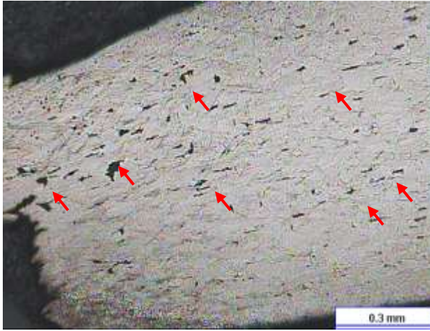
Figure 4 Microstructure at 50X in the region of the fracture surface of steel sheet B. Deformed grains and fracture dimples (red arrows) are observed Source: Prepared by the authors
