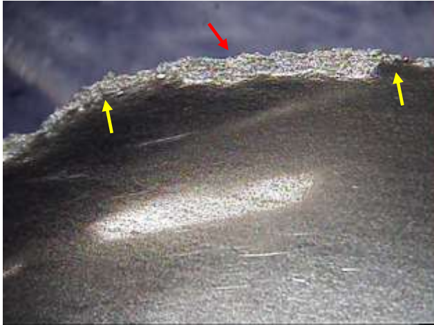
Figure 3 Internal surface of the cracked component after the second deep drawing step. The fracture surface (red arrow) and evidence of plastic deformation (red arrows) can be observed
