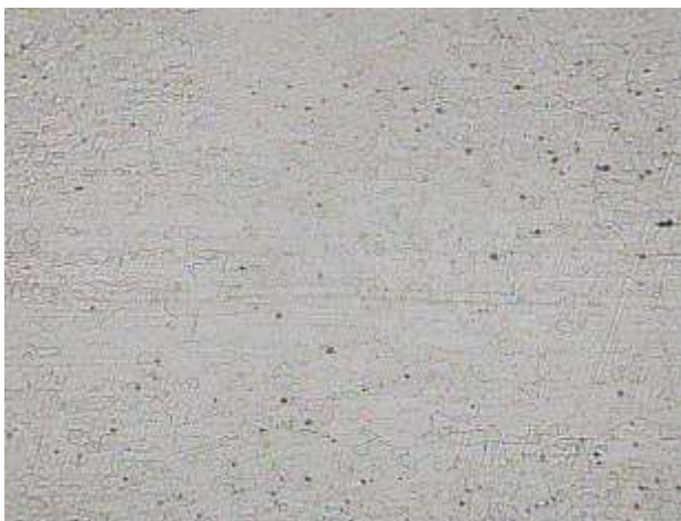
Figure 5 Microstructure at 100X of steel A. Recrystallized grains are observed Source: Prepared by the authors
