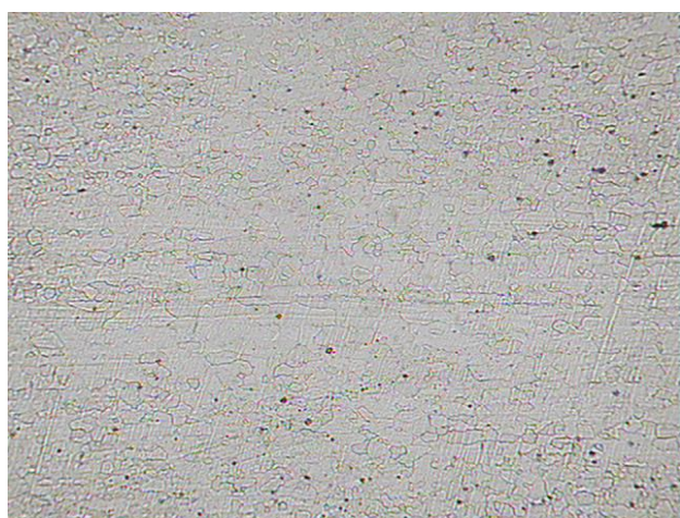
Figure 5 Microstructure at 100X of steel A. Recrystallized grains are observed
