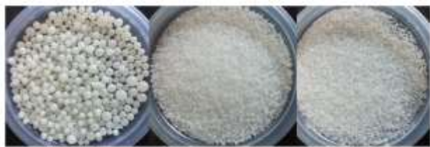
Figure 4 Representative particle sizes at different agitation speeds with PVA3: a) 300 rpm, b) 500 rpm, c) 800 rpm
