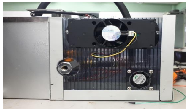
Figure 11 Regulation and cooling system for water in the thermal cycler
