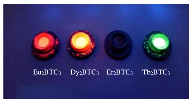
Figure 4 Eu 2 BTC 3 , Dy 2 BTC 3 , Er 2 BTC 3 and Tb 2 BTC 3 MOFs.
