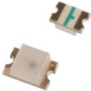
Figure 3 LED surface mount 0805W2C-KHC-B [9]
